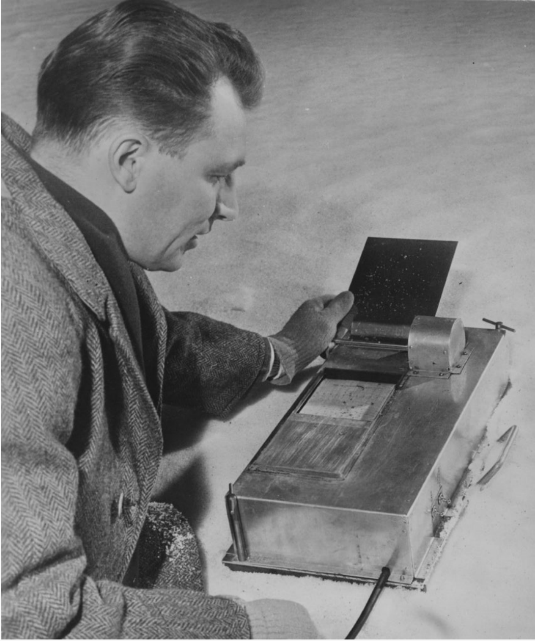
The scientists used this snow crystal recorder to monitor the shape, size and frequency of falling ic crystals.
